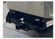
**REAR HITCH**Bolt-on rear hitch
